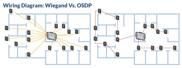
The wiring diagram above depicts how the Wiegand protocol requires homerun cable pulls from the control panel to individual peripheral devices. OSDP is flexible to support either homerun cable pulls or the daisy-chain methodology, depicted on the right.
